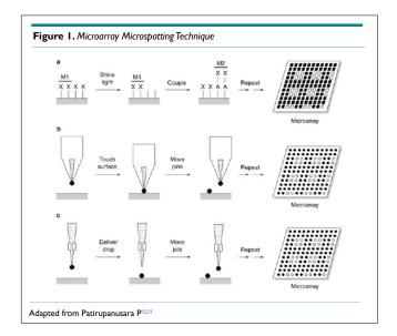
id and hollow (split-open) pen designs are used to transfer target nucleic acid onto the supporting surface. The pen is dipped into the target solution and a small volume of the solution adheres to the pen. When the pen comes into contact with the supporting surface, it transfers a fraction of nucleic acid solution onto solid surfaces (Figure 1).<sup>32</sup>
